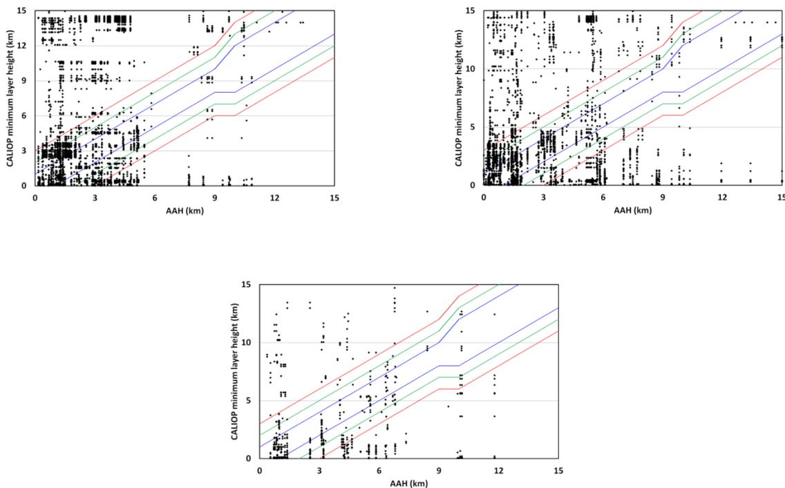
**Figure 7.26. Requirement plots for GOME-2A (upper left), GOME-2B (upper right) and GOME-2C (lower middle). The red, green and blue lines represent the threshold, target and optimal requirements. CALIOP pixels are only shown up to a height of 15 km, which is the detection limit of GOME-2.**
