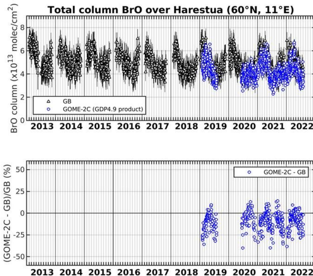
**Figure 7.18. Comparison between GOME-2C GDP-4.9 and ground-based total BrO columns at Harestua (60°N, 11°E). The relative differences appear in the lower plot.**
