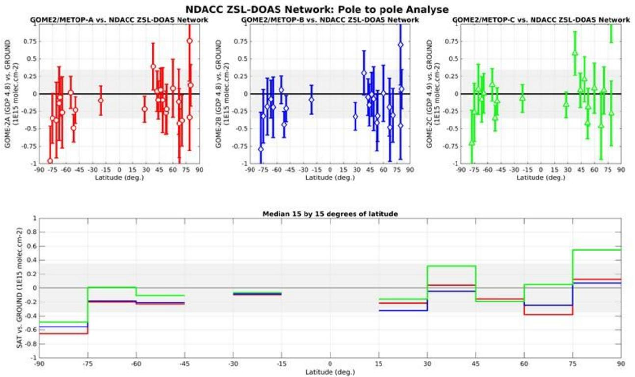
**Figure 7.14.** From pole to pole, median difference between the NO<sub>2</sub> column data reported by GOME-2A/B/C (red/ blue/ green) GDP-4.8 (GDP 4.9 for GOME-2C) and by ground-based ZSL-DOAS spectrometers at about 20 NDACC stations, calculated over 2007 – November 2021 for GOME-2A, 2012 – August 2022 for GOME-2B and 2019 – August 2022 for GOME-2C. Top: median difference at individual stations. Bottom: median difference averaged over 15° latitude bins.
