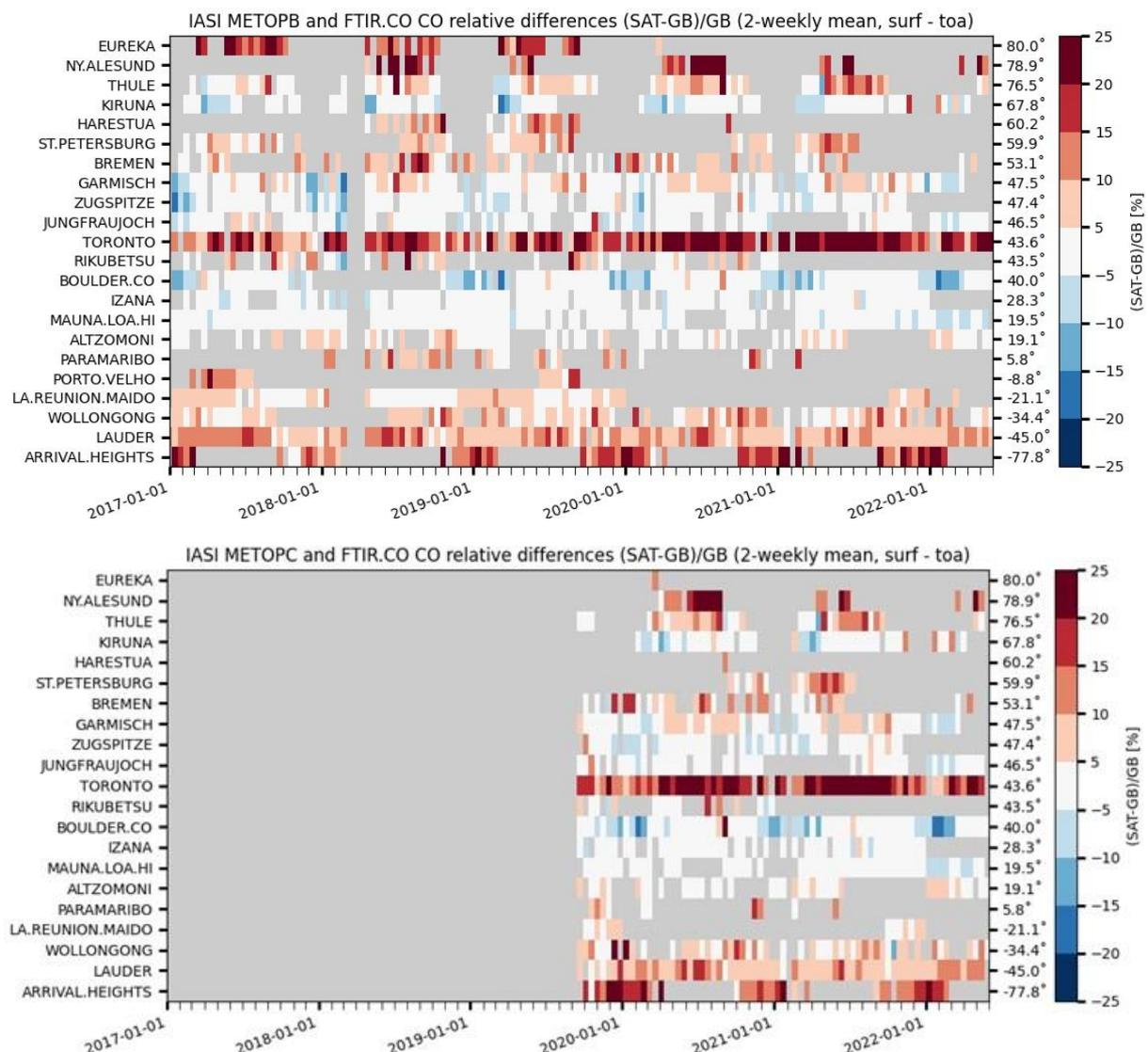
**Figure 7.45. Time-series of bi-weekly relative difference for IASI-B (top) and IASI-C (bottom). Not all stations have co-locations with the Metop-C satellite. The Metop-C relative bias time-series seems to correspond closely to the Metop-B time-series.**
