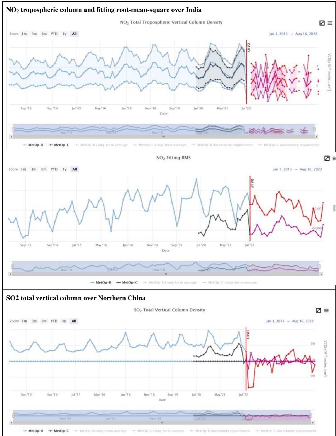
**Figure 7.22. Time-series example for NO<sub>2</sub> and SO<sub>2</sub>, comparing results from GOME-2B and GOME-2C. For GOME-2B, the blue curve shows monthly averaged values, red shows recent daily averages. The black and magenta curves are for GOME-2C.**
