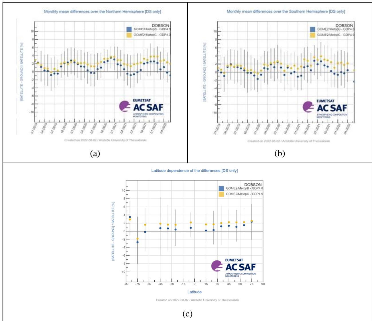
**Figure 7.3.** Panels (a) and (b) show the time-series of the monthly mean percentage differences between GOME-2B GDP-4.8 (blue symbols) and GOME-2C GDP-4.9 (orange symbols) against the Dobson Northern Hemisphere stations (panel a) and the Dobson Southern Hemisphere stations (panel b). Panel c shows the latitudinal dependency of the differences for the Dobson network.
