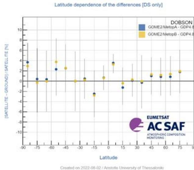
**Figure 7.2. The latitudinal dependency of the differences for the Dobson network.**
