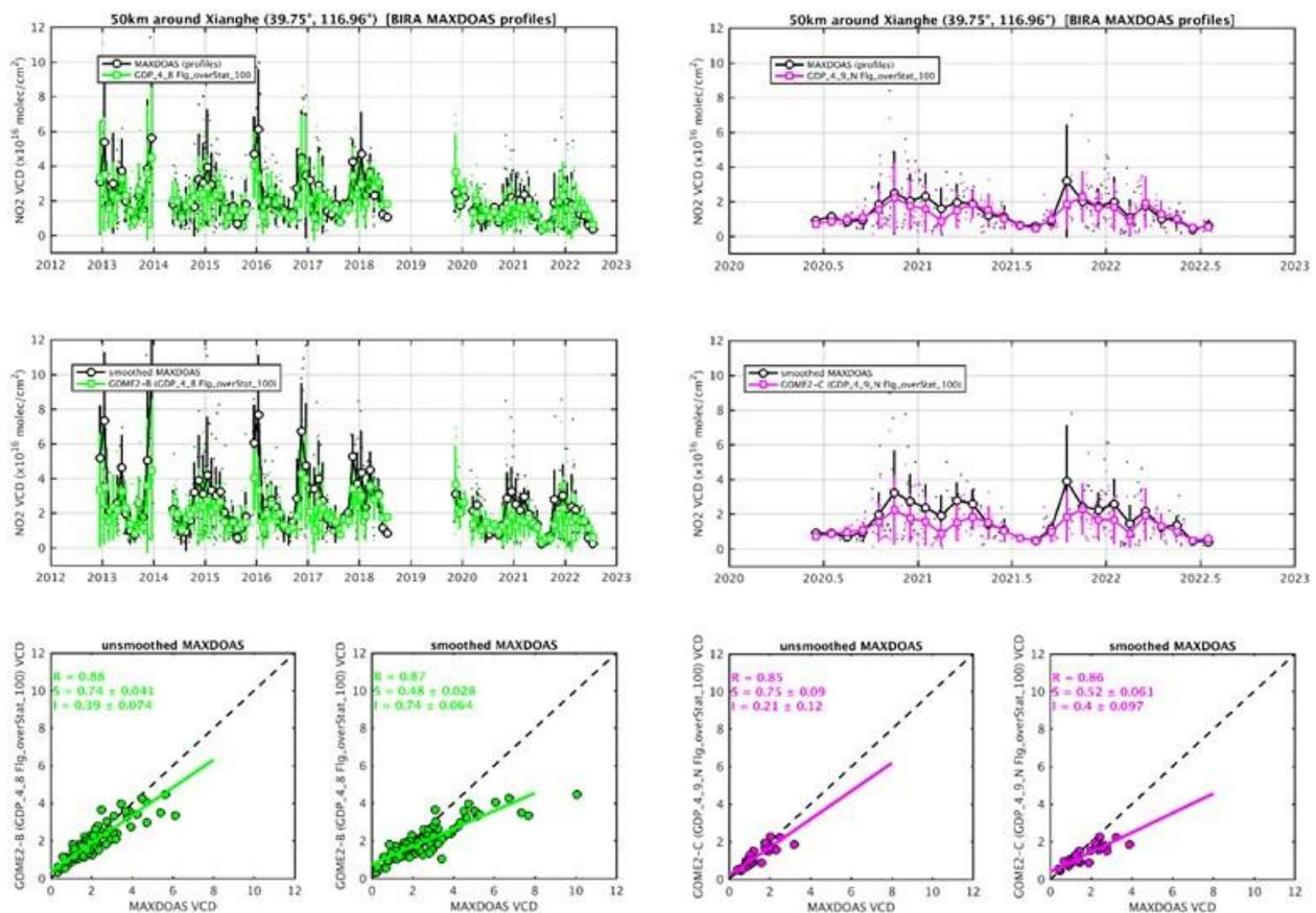
Figure 7.8. Illustration for the Xianghe MAXDOAS versus GOME-2B GDP-4.8 (left) and GOME-2C GDP-4.9 (right) tropospheric NO<sub>2</sub> comparisons, of the application of the satellite averaging kernels on MAXDOAS profiles.
