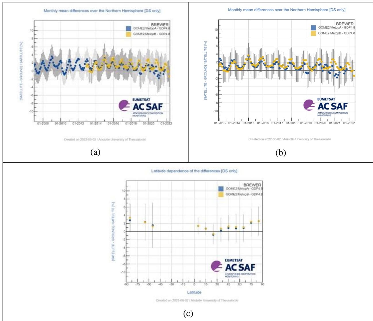
**Figure 7.4.** Panels (a) and (b) show the time-series of the monthly mean percentage differences between GOME-2A GDP-4.8 (blue symbols) and GOME-2B GDP-4.8 (orange symbols) against the Brewer reported TOCs. Panel a shows the full time series of operation for the two sensors and panel b shows the common time period of operation, since 2013. Panel (c) shows the latitudinal dependency of the differences for the Brewer network.
