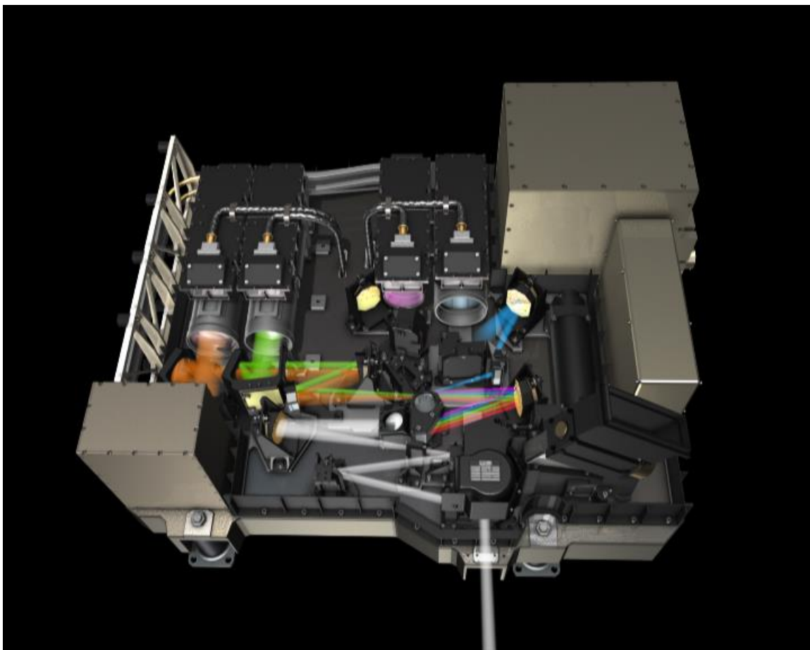
Figure 1: GOME-2 optical layout (courtesy of ESA)
