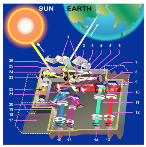
Figure 1: GOME optical layout (courtesy of ESA/ESTEC)
