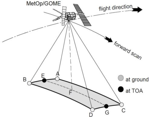
Figure 5: Ground Pixel Geometry
