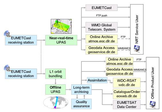
Figure 2: GOME-2/MetOp processing chain
