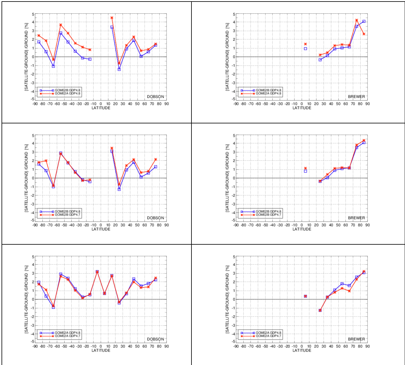
Figure 6.1. Latitudinal dependence of the differences between coincidences between satellite and Dobson [left] and Brewer spectrophotometers [right]. Top row: the effect of the GDP4.8 algorithm on GOME-2A [red] and GOME-2B [blue]. Middle row: GOME-2B comparisons with GDP4.7 [red] and GDP4.8 [blue]. Bottom row: GOME-2A comparisons with GDP4.7 [red] and GDP4.8 [blue].
