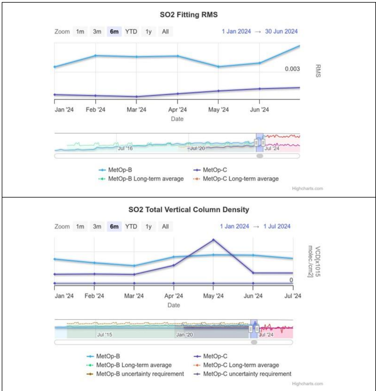
Figure 7.18. The behaviour of the GDP4.8 GOME-2B [blue curve] and GOME-2C [black curve] 6 km plume height SO 2 products between 01/01/2024 and 30/06/2024 over the region of Indonesian volcanoes. Upper panel, the SO 2 fitting RMS is shown and in the bottom panel, the total vertical SO 2 column. The equivalent long-term average is also provided [see insert legend].
